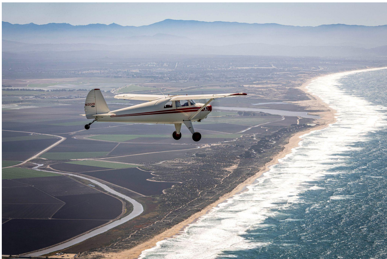
Luscombe N1302B over the Salinas Valley. Note the tail-low attitude in cruise flight and the limited forward visibility compared to a nose-gear airplane.
